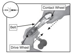
Figure 8. Removing the sanding belt.
